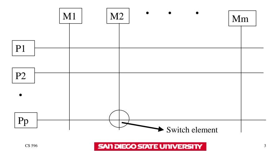
Cross Bar switch is a non blocking network i.e. connection of a processor to a memory bank does not block the connection of any other processor to any other memory bank.
