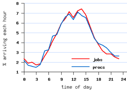
Figure 6. SDSC Blue's load variation by time of day. Graph from Parallel Workloads Archive. [7] Used with permission.
